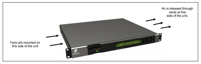
Figure 2.1 Air-flow Through the Equipment
